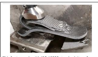
This foot comply with ISO 10328 standard. It performed the following tests: ultimate strength test ( A60, 2415 N), and cycle test (2.000.000 cycles, 1330 N).
