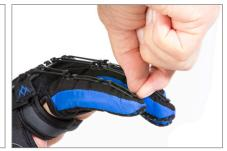
Fig. 32 Reattach DIP Tensioner for all fingers
